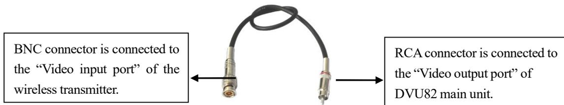
Fig. Video connection line (BNC to RCA) sketch map
