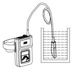
Fig. Immersion disinfection of probe (sketch map)
