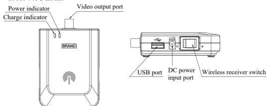
Fig. the charge sketch map for wireless receiver battery
